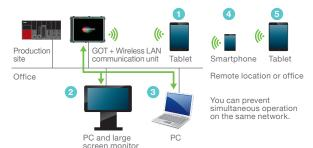
Up to 5 information devices can connect to a GOT at the same time. Multiple maintenance personnel can access the GOT simultaneously to check the status of equipment from different production sites or offices.
