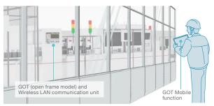
The status of equipment can be monitored using tablets from outside of the clean room or from a remote location.
